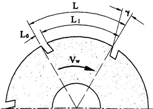
Fig. 1 Schematic drawing of an intermittent grinding wheel
