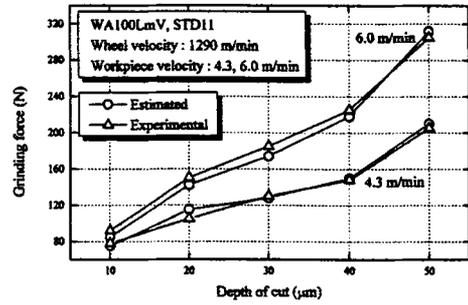
Fig. 5 Result comparison of the simulation and experimentation for grinding force
