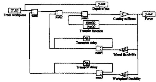
Fig. 3 SIMULAB model of the intermittent grinding process
